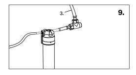
10. Connect hose (4) onto the T adaptor (9) then secure the connection.
