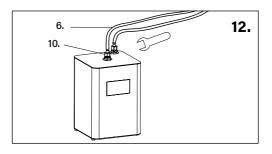
13. Turn on the water supply and do the leakage checking on the water connection. Test systems for leaks, and purge system. Run a minimum of 20 litres water through the tank to remove any air.
