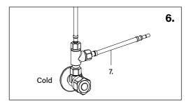
7. Attach the other end of the hose onto filter inlet, then secure the connection.
